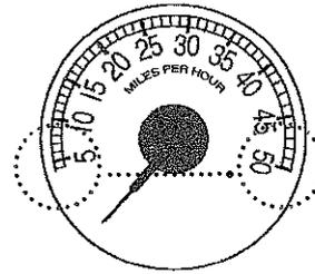
Scale is placed along the upper portion of the circle, which is appropriate for a device that is viewed from above
