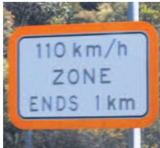
Figure 9. Sign designed to attract additional attention with fluorescent-orange border
