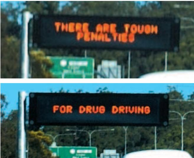
Figure 2. Example of a VMS along the M1
