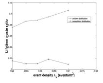
Figure 5. Simulation result for the lifetime waste ratio for uniform and non-uniform deployment strategy, in terms of  $\lambda_s$ , under the conditions of  $\lambda_n=0.02,\ \lambda_t=0.0001\ and\ T_{req}=19 days$
