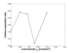
Figure 6. Simulation result for lifetime expectation ratio of non-uniform deployment strategy, in terms of  $\lambda_s$ , under the conditions of  $\lambda_n=0.02,~\lambda_t=0.0001~and~T_{req}=19 days$
