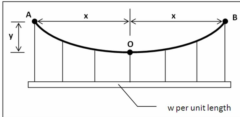
Figure 13. Suspension-bridge cable.
