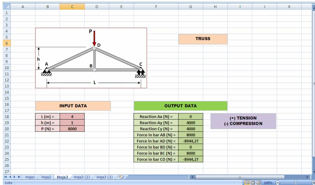
Figure 12. Spreadsheet to solve a particular truss.
