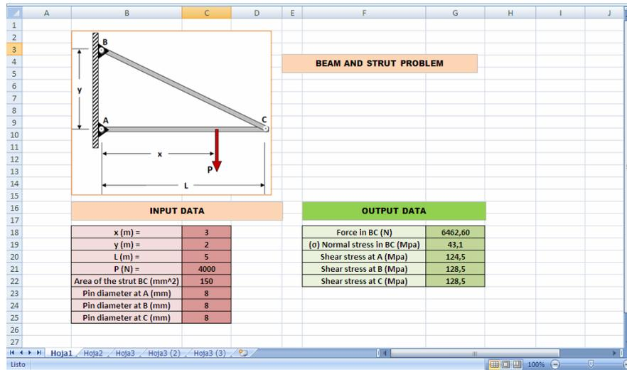
Figure 9. Spreadsheet developed by one of the students.
