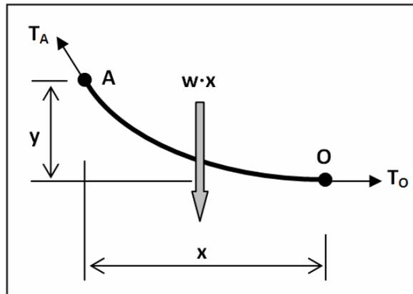
Figure 14. Free-body diagram.
