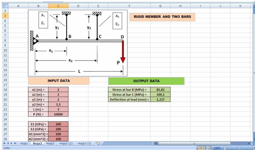
Figure 11. Spreadsheet for a “Rigid member and two bars” problem.
