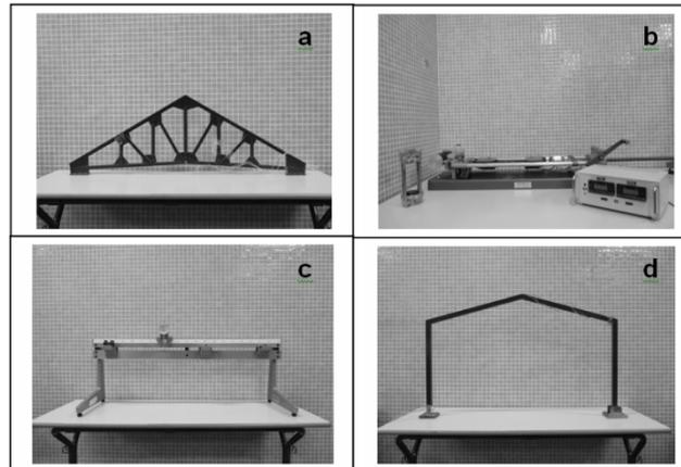
Figure 1. a) Truss, b) Tensometer, c) A system to study deflections in beams, d) Frame.
