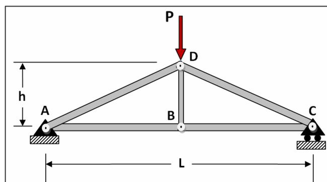
Figure 6. Statically determinate truss.
