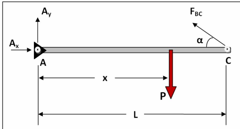
Figure 7. Free-body diagram of the beam AC.
