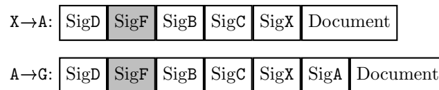
Figure 3.1: A message with broken signatures
