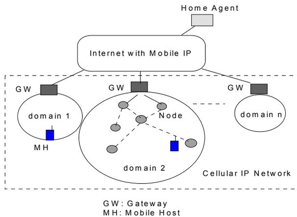
Figure1. Cellular IPv6 network with multiple gateways
