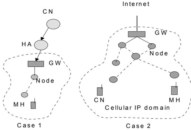
Figure 2: Two cases for IP packets delivery from CN to MH
